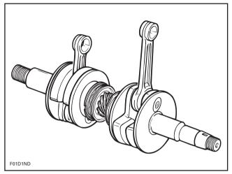
CRANKSHAFT SHOWN WITH CONNECTING RODS
