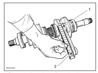
Ruler must be aligned with edge of connecting rod here
