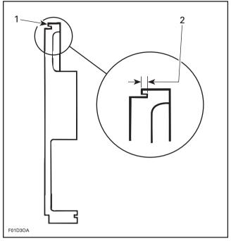
SAME AMOUNT REMOVED FROM COVER SEATING SURFACE AND O-RING GROOVE BASE
