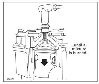
Usually the piston is subject to damage. It may seize or the aluminum on the exhaust side of the piston dome may melt. Pre-ignition is always preceded by detonation.
