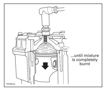
With all operating parameters correct, normal combustion will take place. However, if for some reason the temperature inside the cylinder is increased during combustion, abnormal combustion will occur and lead to serious engine damage.
