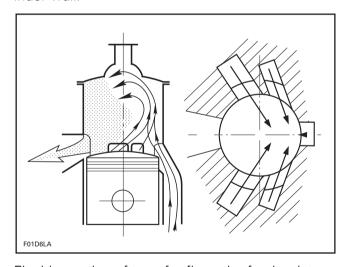
Flushing action of transfer flow; the fresh mixture staying close to the walls of the cylinder expels the burnt gases without mixing with them and/or causing turbulence.
