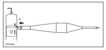
The pipe then bleeds down to approximately atmospheric pressure and the cycle is repeated. The design of the pipe depends upon many factors, including bore, stroke, and desired effective operating RPM.
