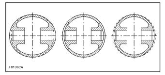
The piston is manufactured out-of-round, the reason being that wrist pin bosses have a greater volume of metal than the other sections of the piston, and consequently, will absorb more heat. The greater the absorption, the greater the area will expand. Under normal operating temperatures, the piston expands and assumes a more rounded shape.
