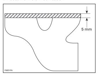
Using a mill, remove 5 millimeters for the cylinder side of the exhaust manifold. The suggested exhaust system is a Factory Pipe using the variable water control system.
