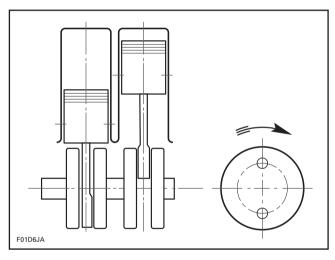
In operation, while 1 piston is at TDC, the other is at BDC, therefore producing a simultaneous ignition and transfer.
